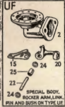
SPECIAL UPPER CASTING FOR TYPE U PUMPS ON BEIFORD AND VADWELL. ALSO SEE LINK ... 1524184. ROCKER PIN BUSH 1524330.
